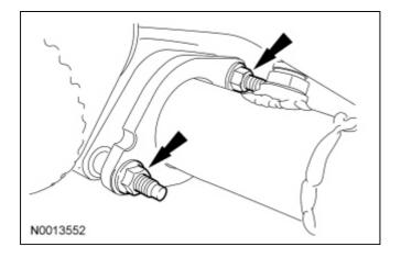
8. Remove and discard the 2 LH catalytic converter-to-exhaust manifold nuts.
